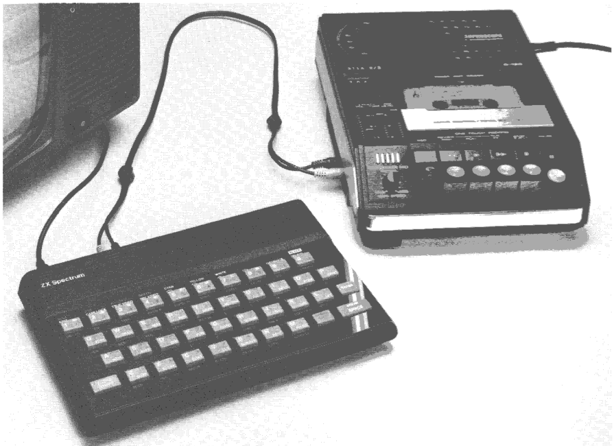
Figure 1.5 A cassette unit attached to the ZX Spectrum.
